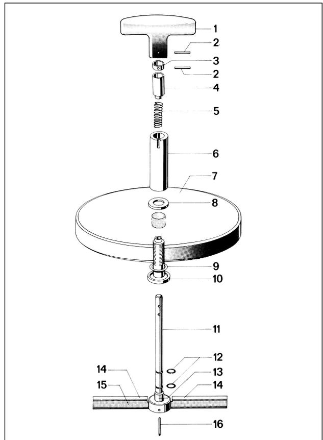
The flexible wiper blades (14) can be easily removed, e. g. when they are worn or damaged, by pressing the T-handle (1) gently against the glass to release the spring pressure. If gaskets (12 or 13) are damaged, they should only be reworked by the manufacturer. Please consult with your supplier.
